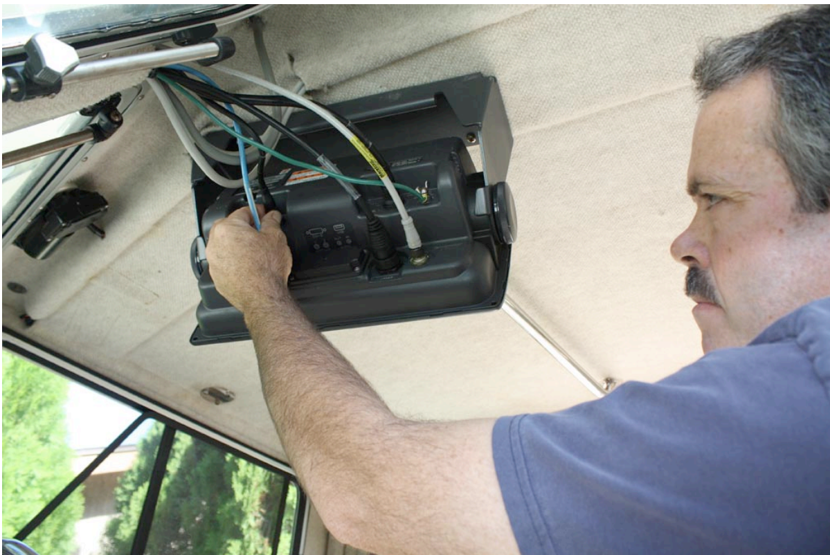
When any piece of marine electronics stops working or you lose functions, check first to make sure no connections have shaken loose
