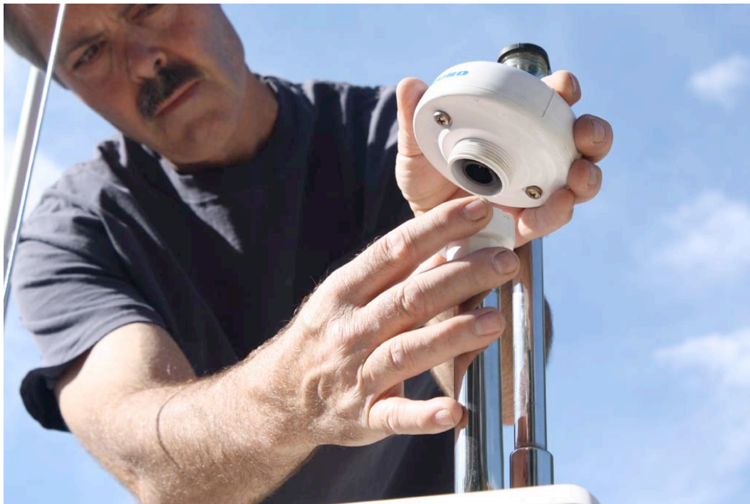
Checking GPS antenna connections should be a first stop when you lose position data
