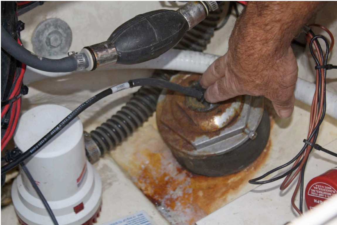
Corrosion and/or frayed transducer cable connections is a common cause of sounder performance issues
